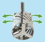
4. The high velocity radially discharged streams impact the slower moving tank flow for additional hydrodynamic shear and circulation, thus ensuring high flow, with no dead spots in the mix tank.
