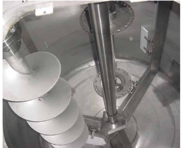
Example of 3-axel Diamix without lifting / lowering
