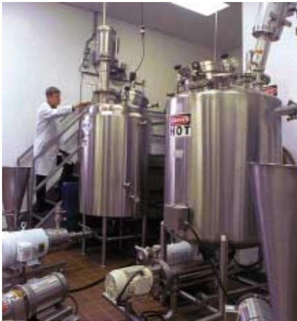
Stainless Rotosolver Dispensers require less horsepower and perform a better mixing job for Richfood Dairy. Source: Admix.
