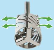
4. The high velocity radially discharged streams impact the slower moving tank flow for additional hydrodynamic shear and circulation, thus ensuring high flow, with no dead spots in the mix tank.
