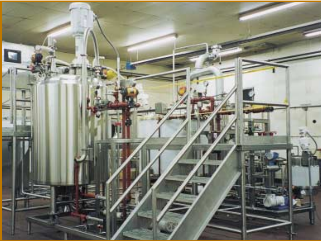
The VacuShear mixer by Admix combines a vacuum delivery system with a high shear blender to produce products with less foaming, aeration and dusting. (Source: A&B Process Systems)
