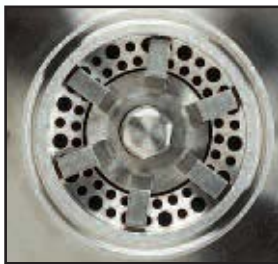
▲ Dual stages: primary axial and secondary radial ▲
