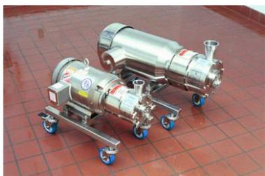
Closed loop continuous flow in-line mixers, as well as those used to recirculate through a batch process, are becoming extremely useful and successful in sanitary processing. In-line high shear mixers are very fast, provide very consistent results, and are very easy to add on to an existing process or production line.
